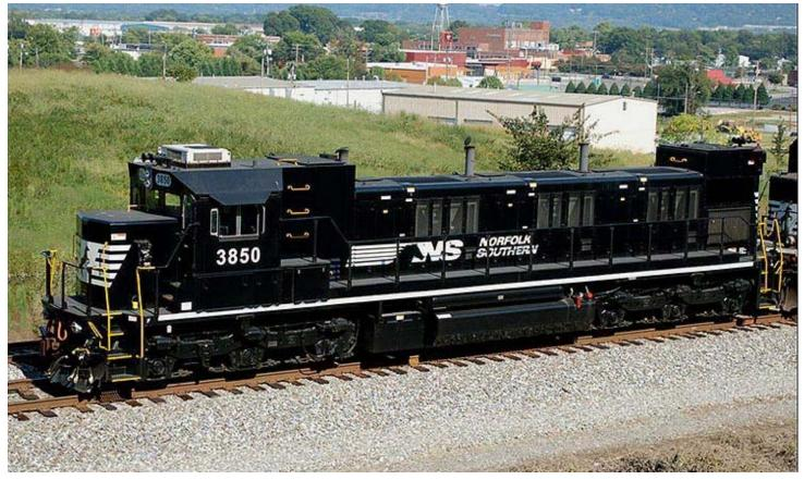
Norfolk Southern #3850 - the first 6-axle genset locomotive delivered to NS. The three-engine 2100hp 3GS21CDE model, built by National Railway Equipment, was sent to Altoona for fine tuning and cab signals and recently was spotted in Manville, NJ, along with NS 100.
