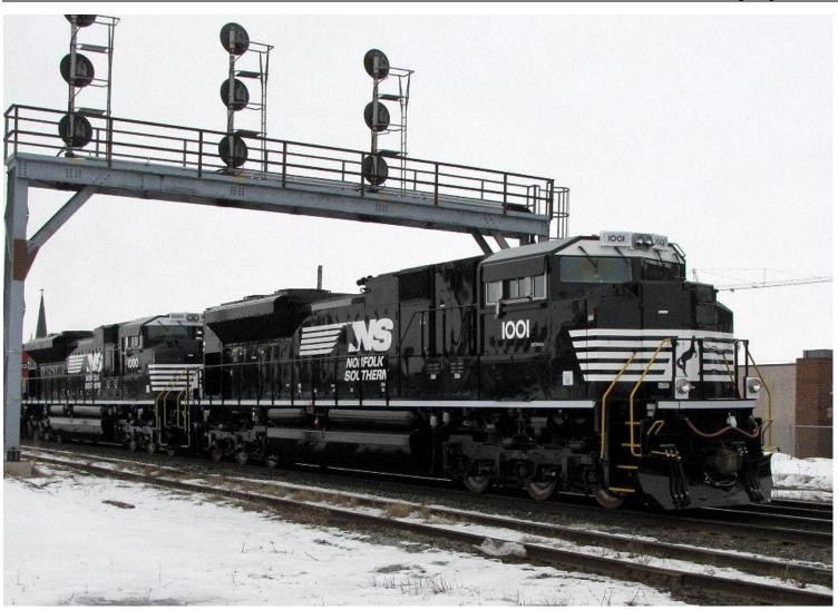
Shown above are NS 1001 and 1000 - two of the 25 new EMD SD70ACE's ordered for this year. The 4300hp. units feature dynamic braking, single controls, cab signals, LSL, air conditioning, and 4900 gallon fuel tanks. They are also set up for Distributed Power operation and for Positive Train Control operation. The new units will be numbered 1000 to 1024. (photo: Geoffrey Williams)
